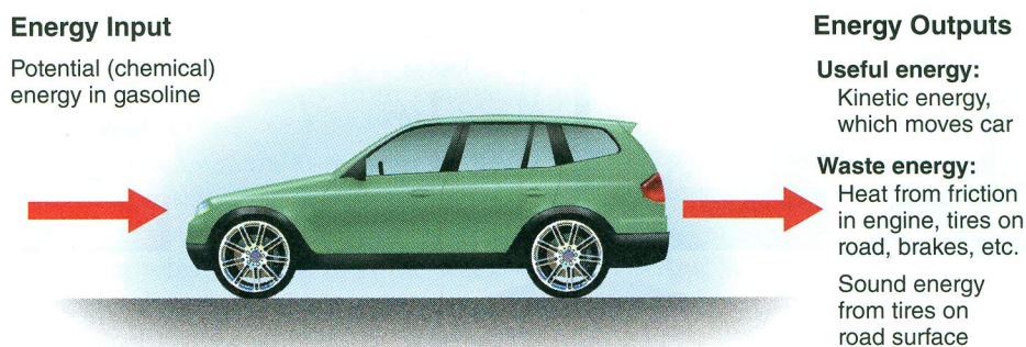
FIGURE 2.13 Conservation of energy within a system. In a car, the potential energy of gasoline is converted into other forms of energy. Some of that energy leaves the system, but all of it is conserved.
